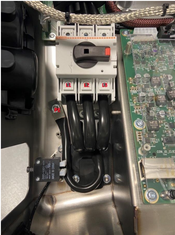
Figure 40: Main switch with connected cables
