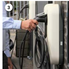
3 Plug in and place the cable over the hook
