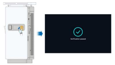
2 If the authentication fails as the card is not activated or gets demagnetized, a failed authentication notification will show on the screen. You can tap **Back** to go to the previous step and select another authentication method.
