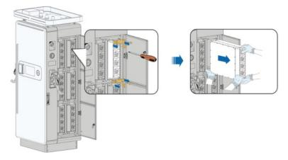
**Step 5** Slowly push the new power unit into the cabinet. Fit the gasket, screws, and wiring terminals back, by performing the above steps in the reverse order.
