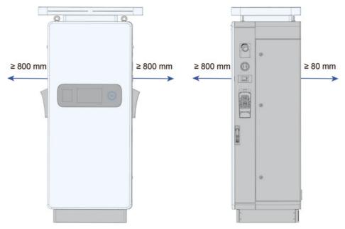
figure 5-1 Space Requirements for Charger Installation
