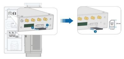
3 Push the SIM card tray gently into the slot until it is in place. Do not exert too much pressure, so as to avoid card deformation or damage.
