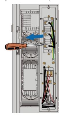
**Step 4** Open the right cabinet door on the charger using the key included in the accessories. Remove the gasket used to fix the power unit. Pull the power unit out of the cabinet by its handles.
