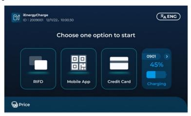
**Step 10** Taking the RFID card as an example, if you choose "RFID", the Energy Star-Ring on the device will blink blue, waiting for you to tap a card over the reader. Upon detecting the card, the system will verify its validity. If it is valid, a successful authentication notification will show up, and you will then go to the interface for charging connector selection.
