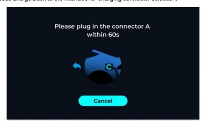
**Step 2** Plug in the connector before the end of the countdown. Upon detecting that the connector is plugged into the port, the system will go into the preparation process. You will see the below interface. By tapping **Cancel**, you can guit the process immediately.
