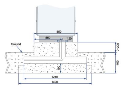
figure 5-2 Foundation Dimensions (mm)
