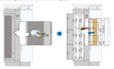
Step 3 Remove the screws and wiring terminals connected to the power unit.
