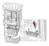
**Step 4** Trim the seal to make an opening, which should be done properly according to the outer diameter of the AC cable.
