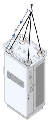
Step 2 Hoist the charger vertically and smoothly. Make sure it is always held steady and does not tilt.
