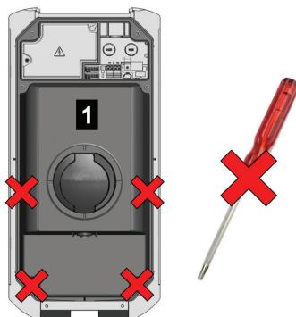
Fig. 1-1: Screws on front part
