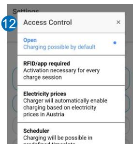
2. RFID/app: charging process needs to be enabled by the slider "Activation" (2) or RFID.
