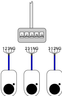
When installing several chargers, connect the phases of the first, second and third charger to the house circuit in rotation, as shown in the adjacent figure, in order to obtain an even load balance when charging single-phase vehicles.
