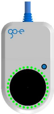
The charging process is terminated by the vehicle. This is usually the case when the vehicle's battery is fully charged. The cable remains locked (default settings) in the type 2 socket after the charging process is complete until it is removed from the vehicle (theft protection).
