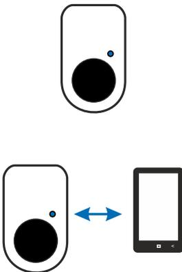
This means you can already control the Charger locally via the built-in hotspot.
